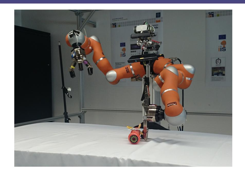
Introducing corrective actions in a pushing task is possible by sensing. Control parame-
