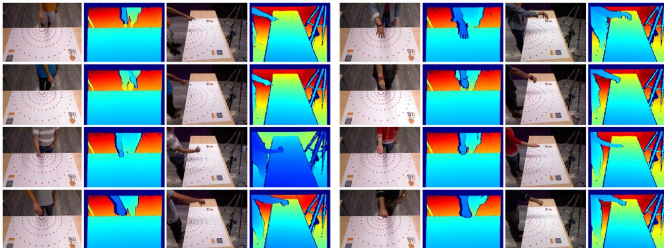
Gestures recorded from frontal and side view. *T-B*: Finger pointing, Tool pointing, Thumb up (approve), Thumb down (disapprove), Grasp open, Grasp close, Receive, Fist (stop).
