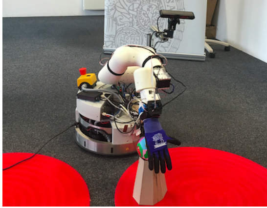
Fig. 1: SQUIRREL robot with the SoftHand as an end effector.
