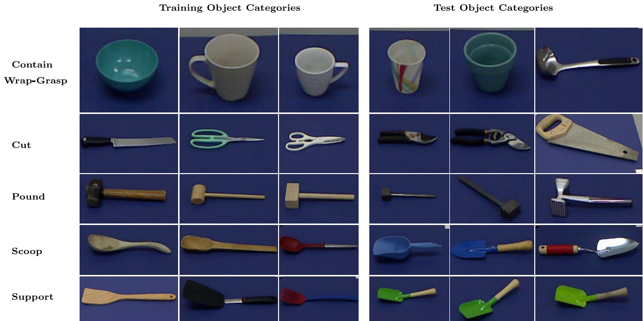
Fig. 8 Examples of training and test objects used for affordance detection on novel object categories in Fig 7. For simplicity up to two instances of each category are shown. All objects with handles are labeled with the grasp affordance. For the test object categories tenderizer and shovel, two views of the same instance are shown in the fourth and fifth columns.
