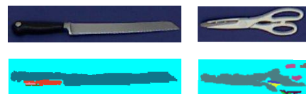
Fig. 10 Segmentation error for patches. Top row: RGB image of objects; bottom row: segmented patches based on Region Growing Segmentation. Each patch is shown in a different color. Patch segmentation uses surface normals of adjacent points. This results in a false segmentation in disconnected areas or areas with too few points.
