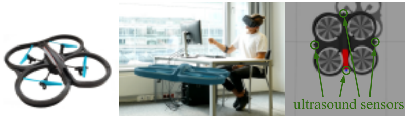
Fig. 1: Quadcopter (left), gesture-based control, here with MYO bracelet, Oculus Rift (middle), Gazebo drone model, with virtual ultrasound sensors (right).
