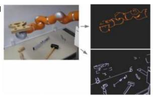
enforced by probabilistic inference. In the spirit of traditional articulated models, those constraints are modeled in a Markov random field, and an algorithm such as belief propagation can then identify a globally consistent result for the pose of all links.
