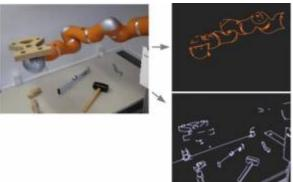
articulated links are enforced by probabilistic inference. In the spirit of traditional articulated models, those constraints are modeled in a Markov random field, and an algorithm such as belief propagation can then identify a globally consistent result for the pose of all links.
