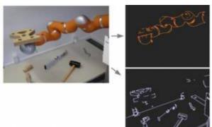
articulated links are enforced by probabilistic inference. Similarly to the traditional articulated models, those constraints are modeled in a Markov random field, and an algorithm based on belief propagation can then identify a globally consistent result for the configuration of all links.
