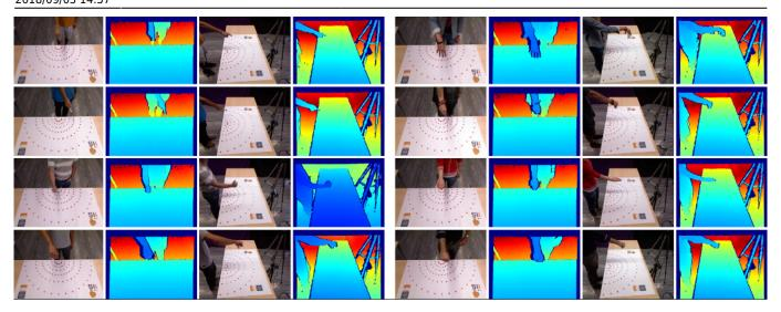
Gestures recorded from frontal and side view. *T-B*: Finger pointing, Tool pointing, Thumb up (approve), Thumb down (disapprove), Grasp open, Grasp close, Receive, Fist (stop).
