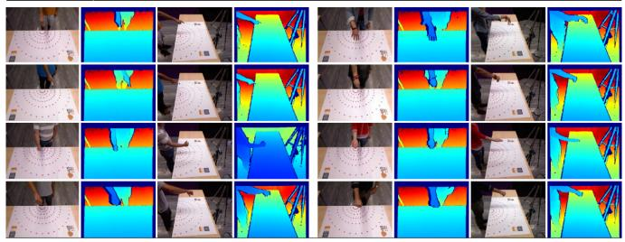
Gestures recorded from frontal and side view. *T-B*: Finger pointing, Tool pointing, Thumb up (approve), Thumb down (disapprove), Grasp open, Grasp close, Receive, Fist (stop).
