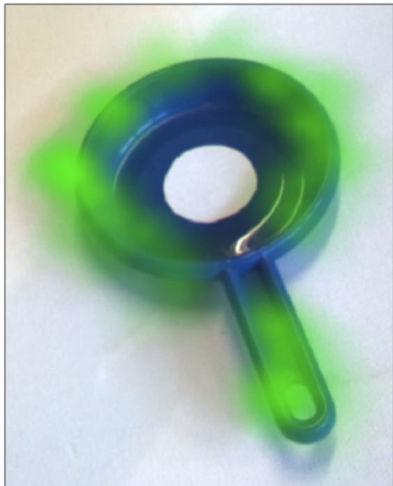
Projection of a 6DOF grasp density on a 2D image. Grasp success likelihood is proportional to the intensity of the green mask.
